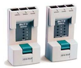
Unique snap-together two piece design allows for testing installed cables easily. The Master unit applies a test voltage to the pairs of either 568A, 568B or USOC 4 pair cables. The Remote unit then displays the corresponding green (straight through) or red (crossed over) results on its LEDs. No lights indicate open pair. 9V battery included. One year warranty.
